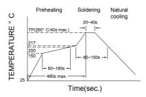
Figure 1. Re-flow Soldering
